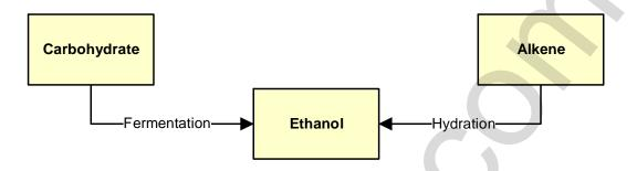
Ethanol is globally produced on a large-scale by two main processes as shown on the flow chart.
