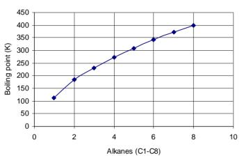
The graph shows the boiling points of the alkane series from methane to octane.
