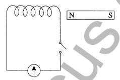
The switch is then closed and the magnet is moved towards the coil and then back away from the coil. This action is then repeated. The galvanometer indicates that a current is induced within the coil. If the electromotive force (emf) is plotted against time a graph as shown below is obtained.
