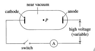
When the circuit is switched on, which field(s) then exist at point P?
