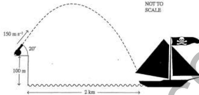
An enemy ship was sailing 2 km from the coast. A cannon on a 100 metre-high cliff fired a canon ball at an angle of  $20^\circ$  to the horizontal, at speed of 150 m/s.
