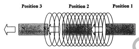
Which of the following graphs best represents how the emf generated in the coil changes as the bar magnet moves from position 1, through 2, to 3?
