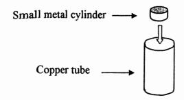
Yet a small magnet of identical dimensions takes much longer to fall through the tube.
