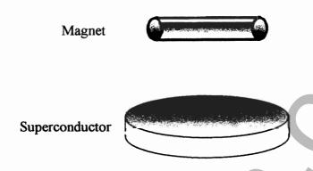
(b) In 1933, two German physicists, W Meissner and R Oschenfeld, found that after a superconducting material is cooled below its critical temperature, and a magnetic field is applied, the material expels all magnetic flux from its interior.
