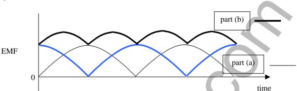
Most students answered the first part well showing that the emf is reversed each half cycle by the commutators.
