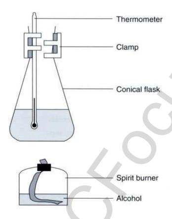
Methanol, ethanol and 1-propanol were burned in separate spirit burners and used to heat a container of water. The volume of water heated by each alkanol was 100.0 ml.
